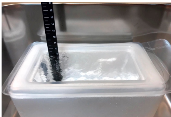
Figure 8. Filling the N-Sleeve with Liquid Nitrogen inside the N-Sleeve
